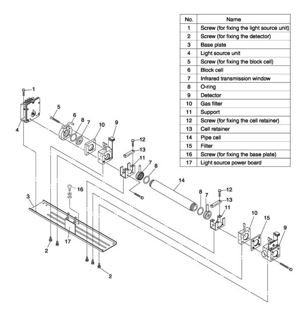
Figure 7-3: Measuring Unit with 2-Component Block and Pipe Cell
